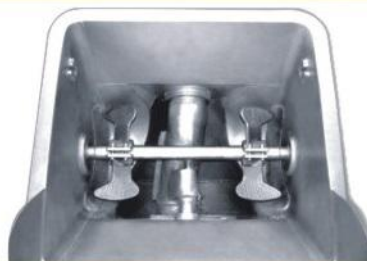
摆动及搅拌机构：采用动压双层密封及隔离漏浆设计。 Swing and mixing mechanism with double layer sealing and isolated leakage device.
